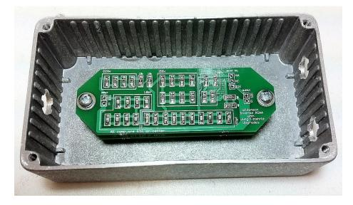
*Figure 4 - Two boards are stacked one upon the other with 5mm spacers to create a stereo IRN*
